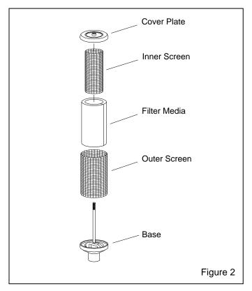
**5.1.1** The inlet filter ensures that no foreign particles enter the pump inlet. A dirty filter restricts air flow, and if not corrected could lead to possible motor overload, poor performance and early pump failure.
